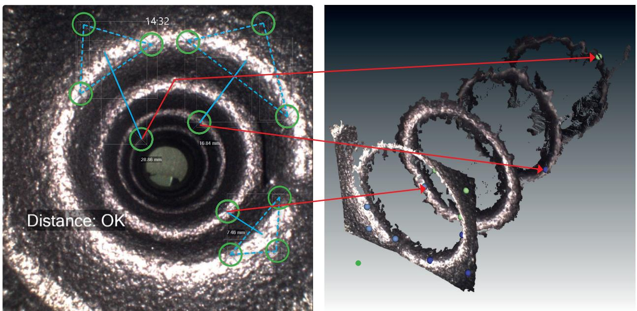
High resolution 3D- view of color image and measurements, making part inspection and measurement verification very easy.
